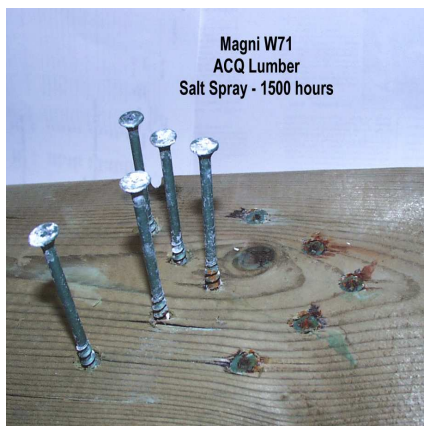
Figure 3: W71 – Salt spray
